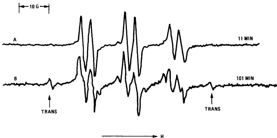
Fig. 5. Typical ESR spectra of the spin labels in the TGDDM-DDS-PBN system; curing temperature = 140°C.
